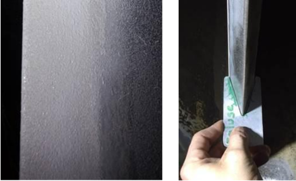
Figure 14. Photograph of artificial sand roughness applied at the trailing edge of the stiffener plate AA as temporary solution (left) and final trailing edge profile with 30° angle after trailing edge site grinding as long-term solution (right).
