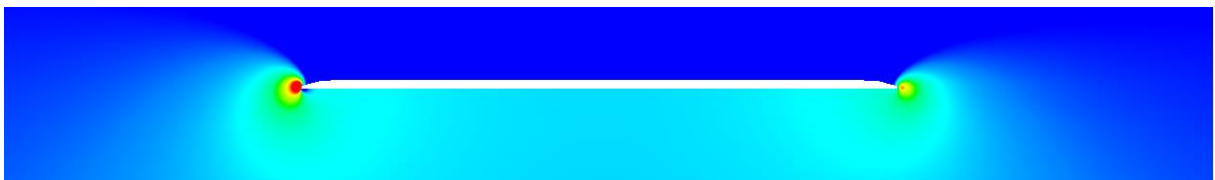
Figure 8. Unsteady pressure field obtained with 2D CFD of the flow around the stiffener “BB”.
