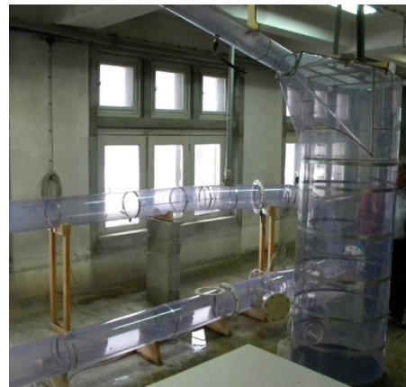
Fig. 9. Scaled hydraulic model of the surge tank ST2 connected to head race tunnel model
