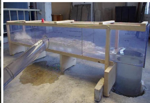
Fig. 5. Top: Laboratory test rig. Bottom Left: scaled hydraulic model of original surge tank ST1. Bottom right: scaled model of surge tank upper tank
