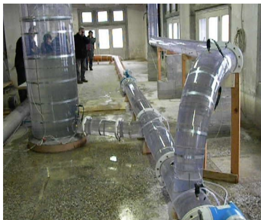
Fig. 9. Scaled hydraulic model of the surge tank ST2 connected to head race tunnel model
