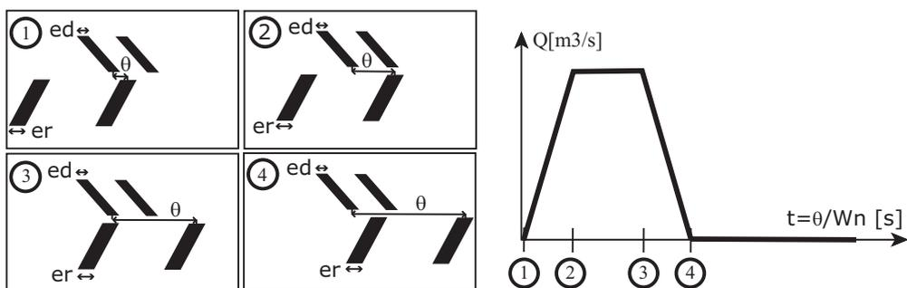
Figure 6 Idealized discharge evolution between a impeller vane and a guide vane as function of the spatial coordinate of the impeller  $\theta$ .
