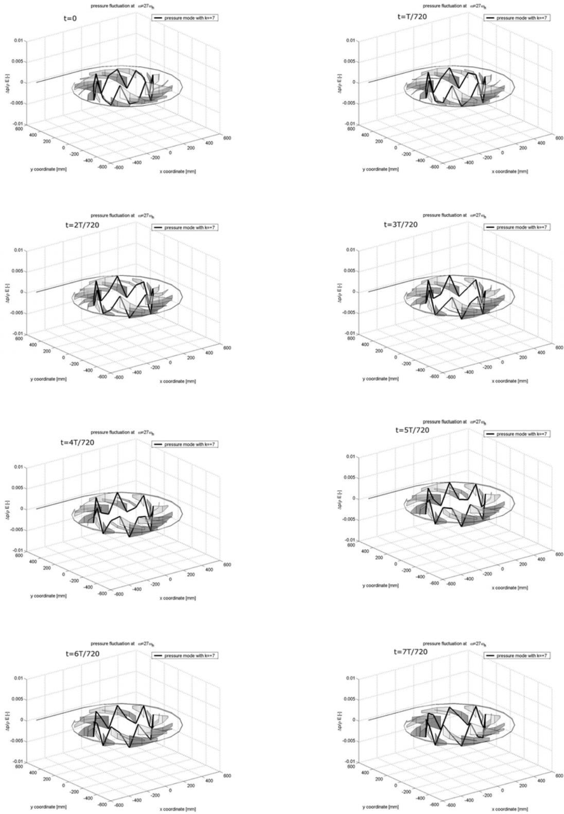
Figure 14 Pressure fluctuations patterns for  $k_1 = +7$ ,  $f/f_b = 27$  in the stationary part,
