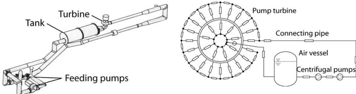
Figure 9 EPFL test rig PF3 and hydroacoustic model of the closed loop test rig N°3.
