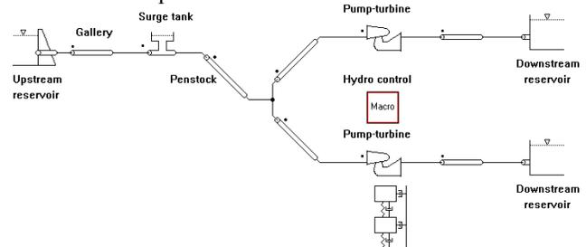
Fig.2. Hydraulic system of the power plant
