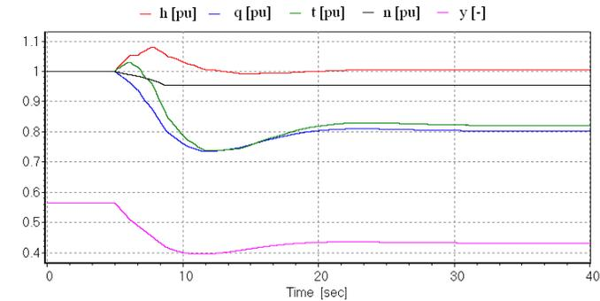
Fig.18. Transient behaviour of the pump-turbine in (pu)
