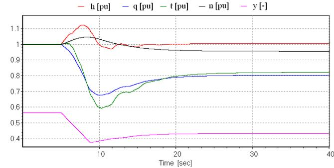
Fig.24. Transient behaviour of the pump-turbine in (pu)
