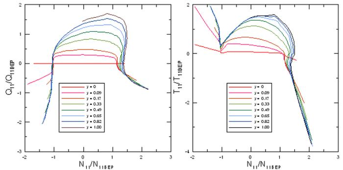
Fig.3. Pump-turbine characteristics
