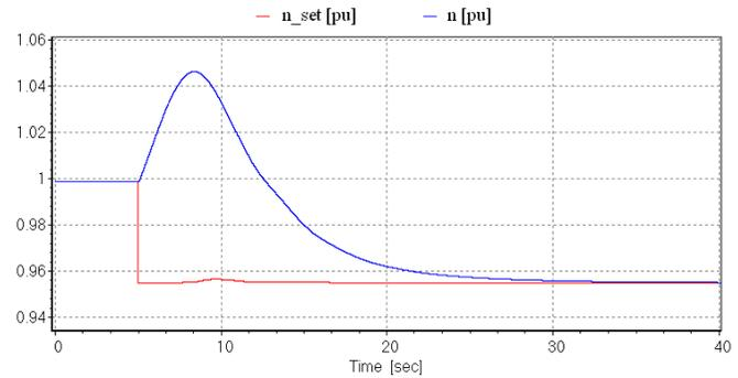
Fig.23. Speed set point (red) and speed (blue) in (pu)
