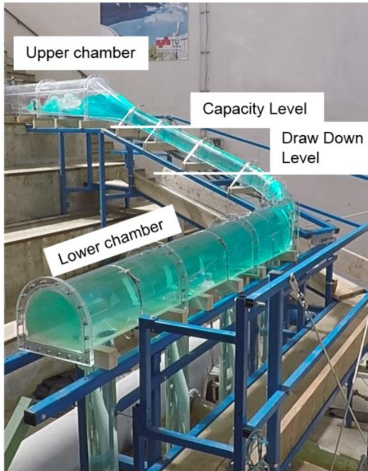
Fig. 2: Tail race surge tank model test
