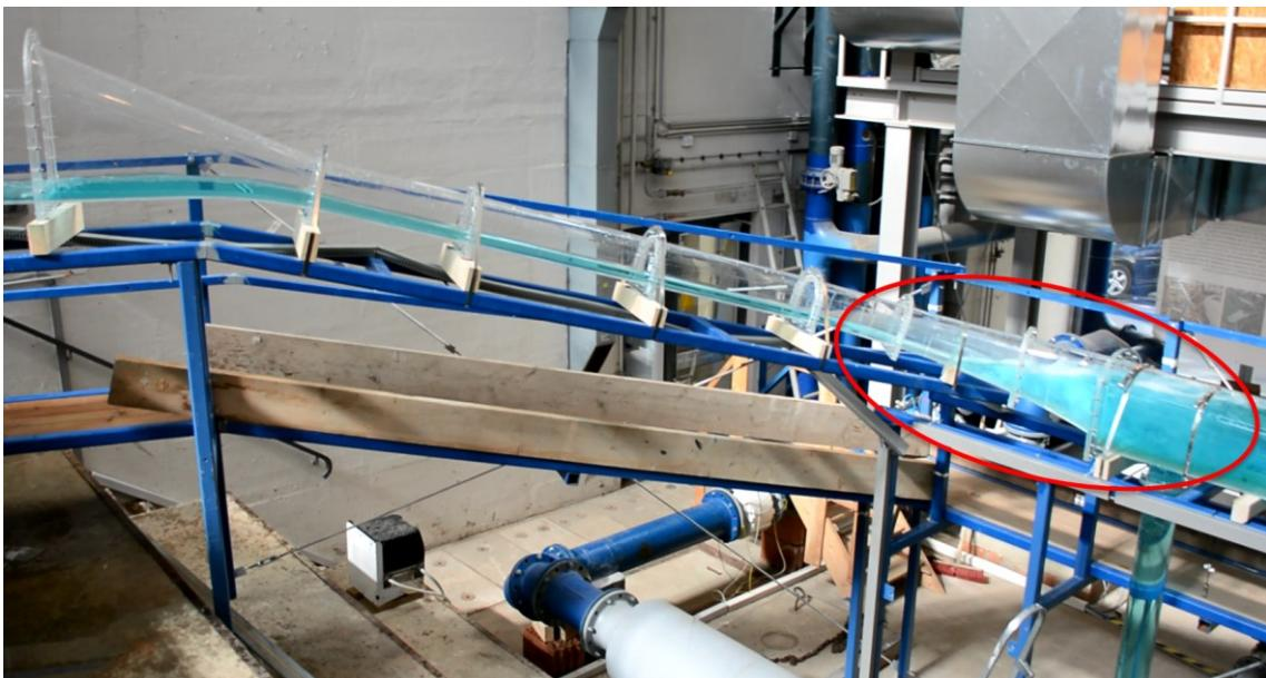
Fig. 8: Massive air intrusion in the lower chamber without measures before optimization
