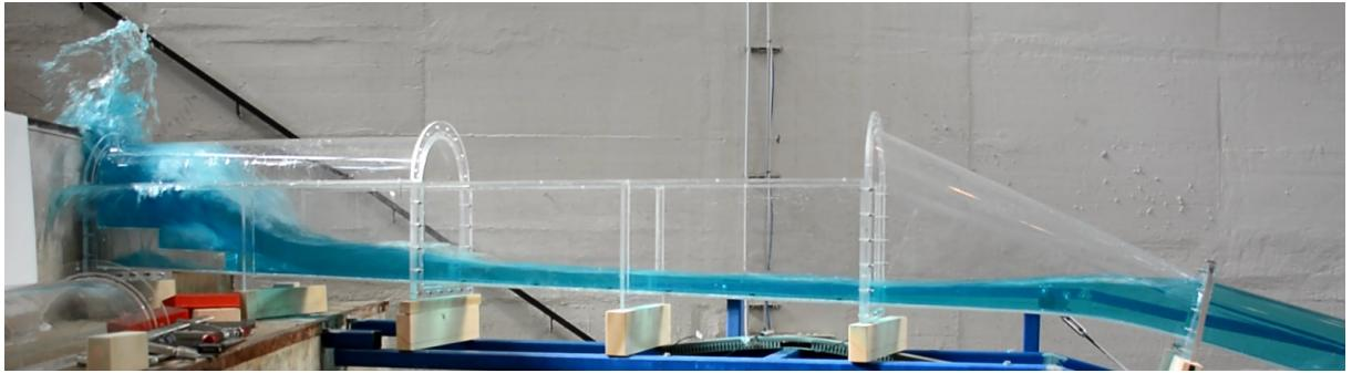
Fig. 3: Upper chamber surge without dissipation structures before optimization
