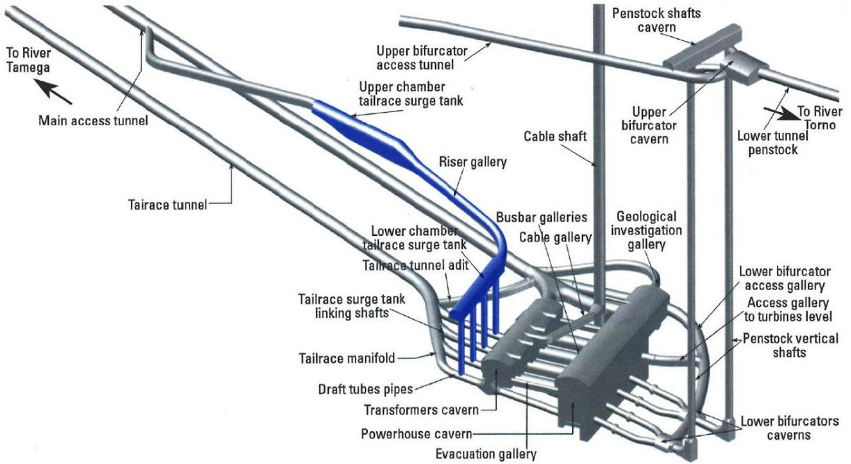
Fig. 1: Power cavern, civil works and tail race surge tank indicated [1]
