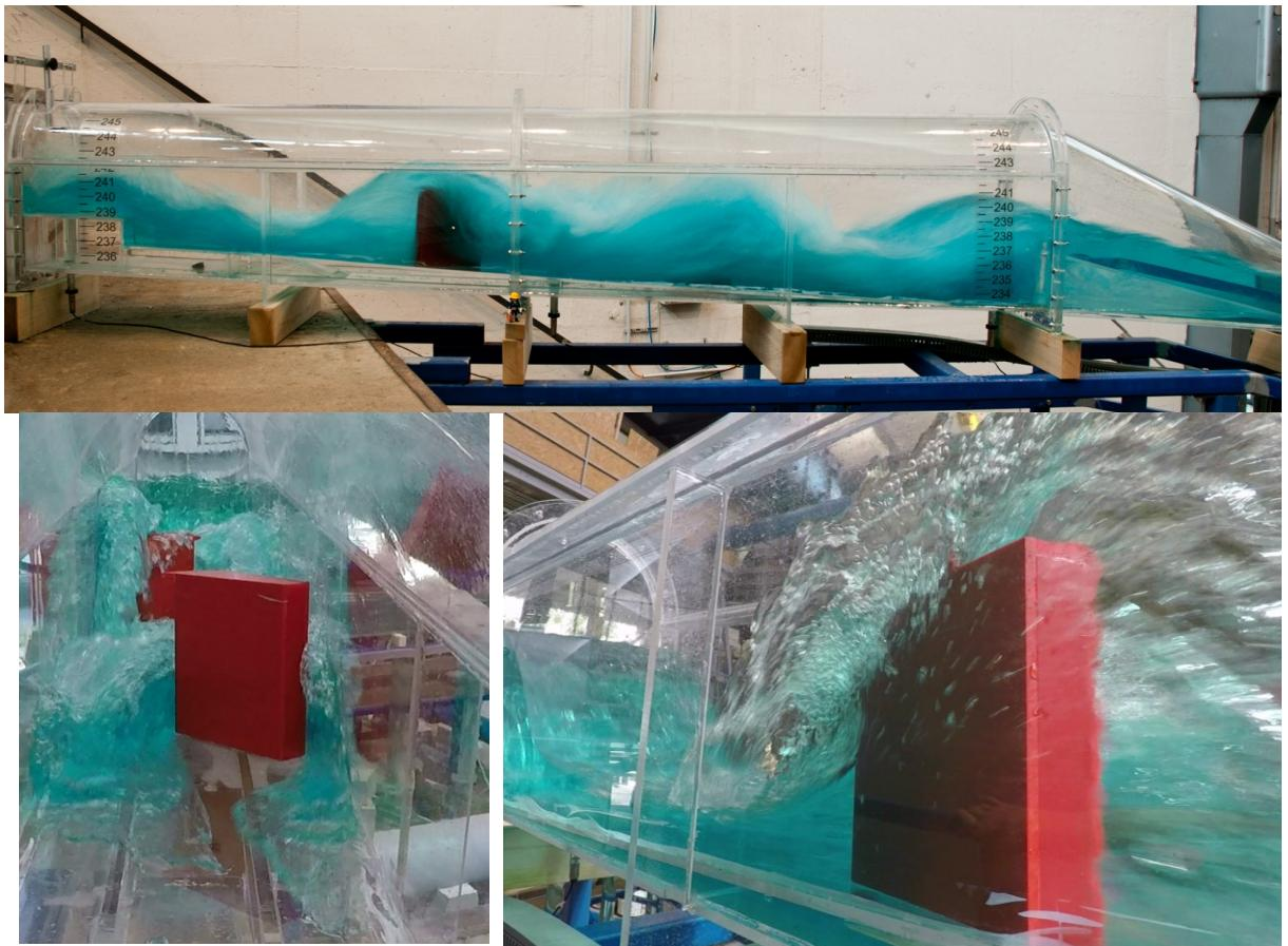
Fig. 4: Upper chamber surge final solution with dissipating structure
