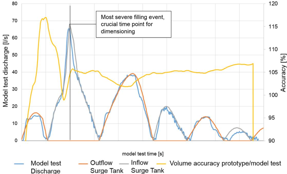
Fig. 5: Comparison model test inflow of model test, scale factor of time 5 [-]
