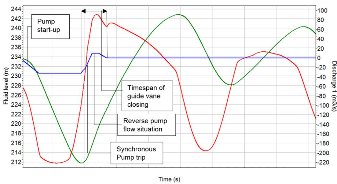
Fig. 7: Load case A, 1D numerical mass oscillation for most unfavourable synchronous pump trip, discharge imposed boundary condition (WANDA 1D software)
