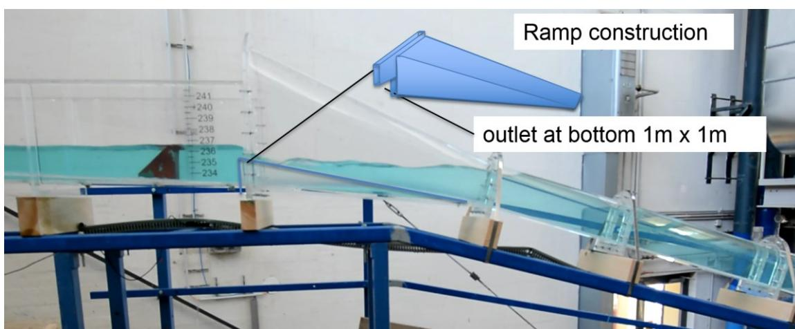
Fig. 9: Ramp construction that traps the water as solution to effectively separate and dampen the outflow of the upper chamber to prevent large air intrusion
