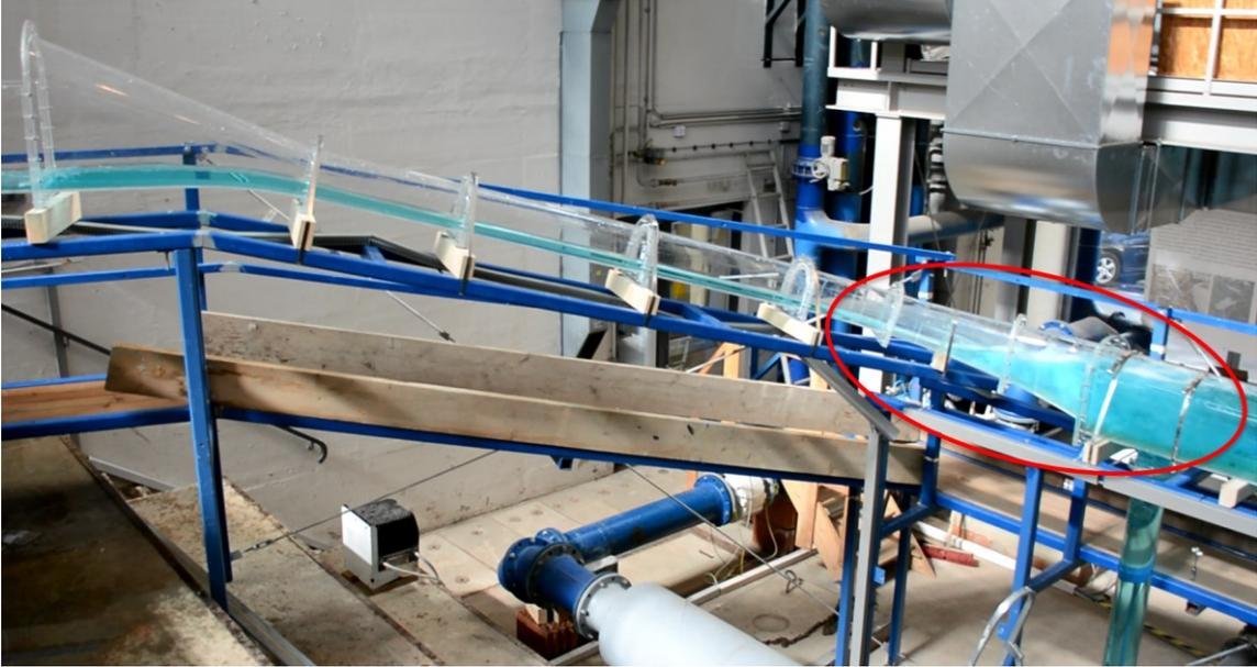
Fig. 8: Massive air intrusion in the lower chamber without measures before optimization
