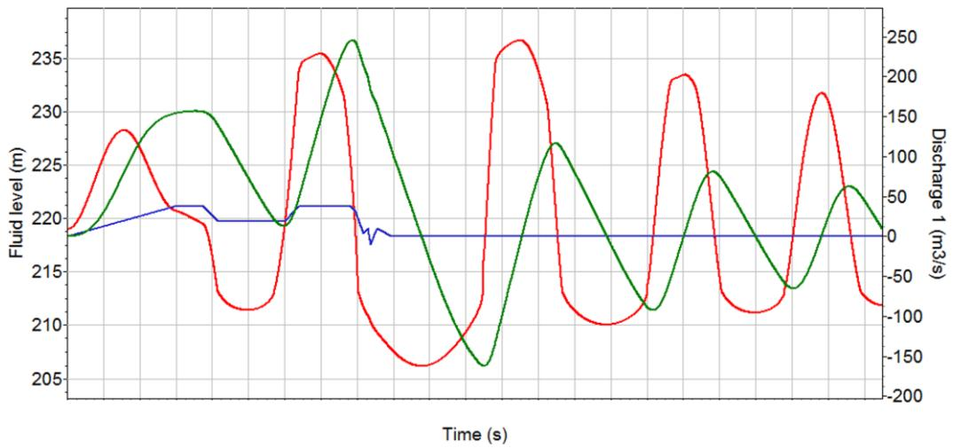
Fig. 6: Load case B, 1D numerical mass oscillation simulation for lowest level in lower chamber, level 205 m a.s.l. is the bottom of the lower chamber (WANDA 1D software)
