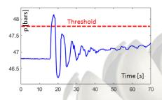
Type 1: Exceedance of the admissible limit of a measured quantity
