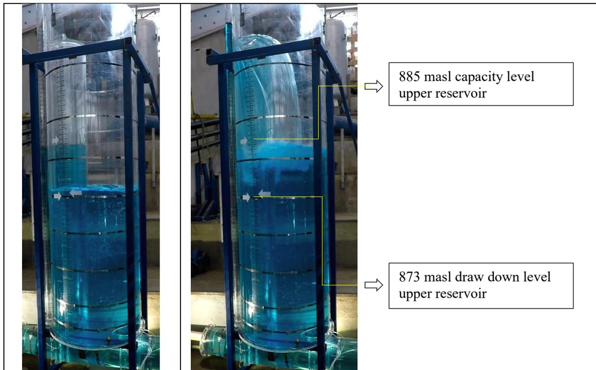
**Figure 9.** Examples of Gouvães headrace surge tank transient flow achieved during physical transient model tests at TU Graz for the critical exceptional load cases related to upsurge with water fall, starting levels are indicated.
