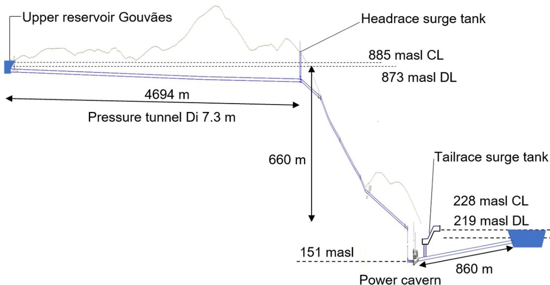
**Figure 1.** Waterway layout of the Gouvães 880 MW PSPP.
