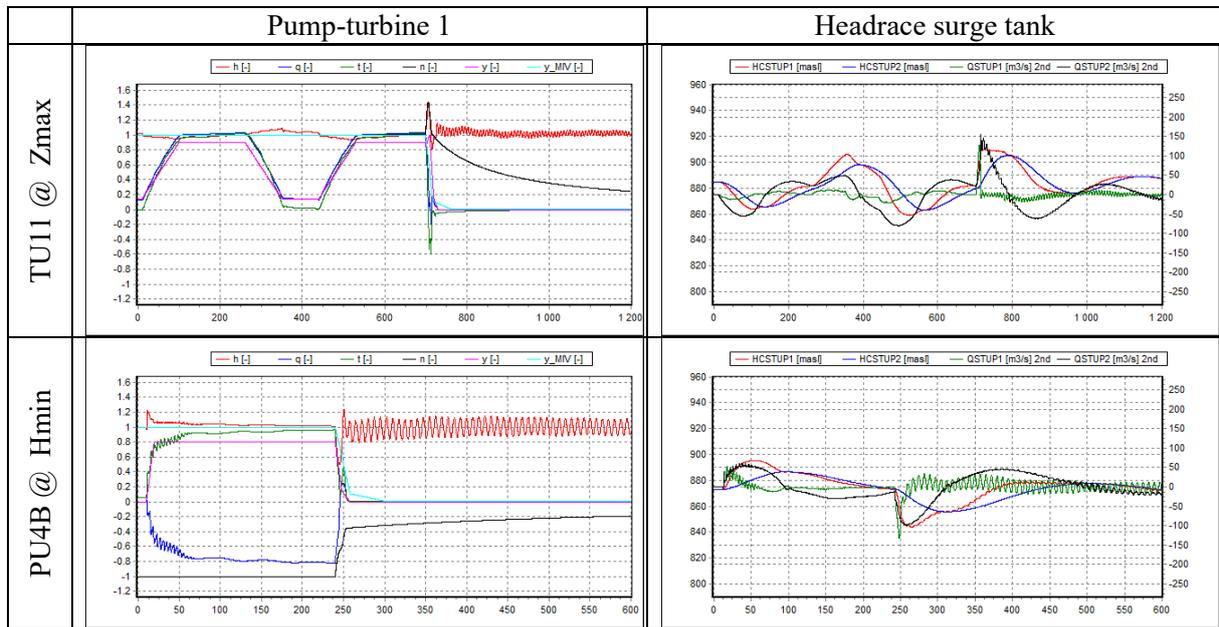
**Figure 7.** Numerical simulation results of the transient behaviour of the pump-turbine 1 and headrace surge tank related to critical **exceptional** load cases for the headrace surge tank maximum (top) and minimum (bottom) transient water levels.
