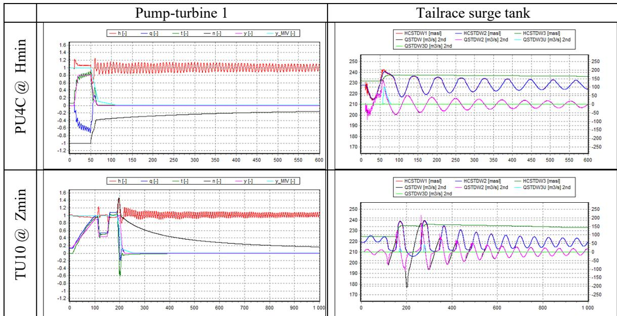
**Figure 8.** Numerical simulation results of the transient behaviour of the pump-turbine 1 and tailrace surge tank related to critical **exceptional** load cases for the tailrace surge tank maximum (top) and minimum (bottom) transient water levels.
