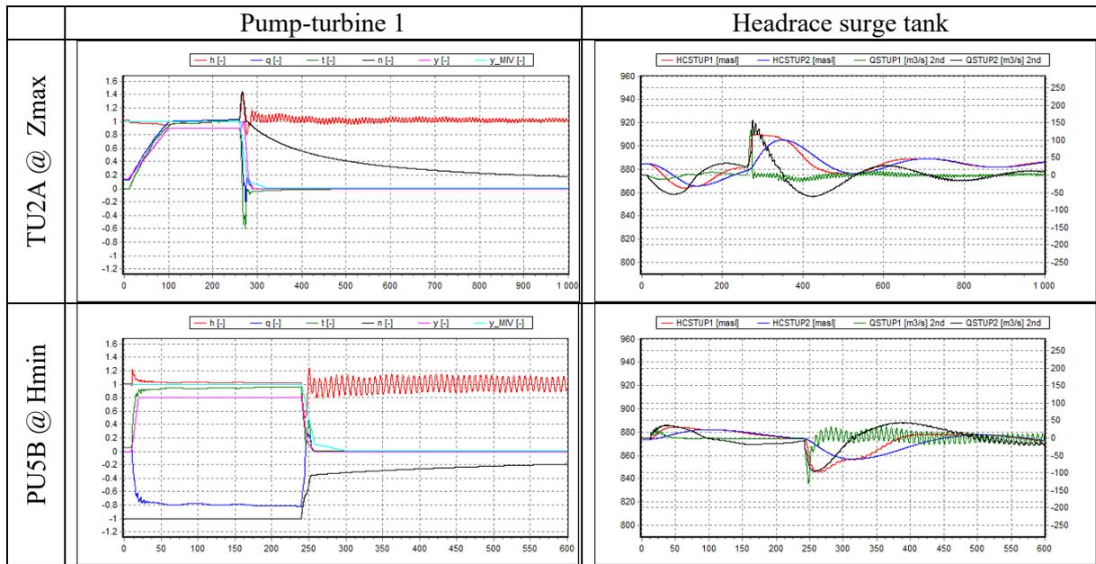
**Figure 5.** Numerical simulation results of the transient behaviour of the pump-turbine 1 and headrace surge tank related to critical **normal** load cases for the headrace surge tank maximum (top) and minimum (bottom) transient water levels.
