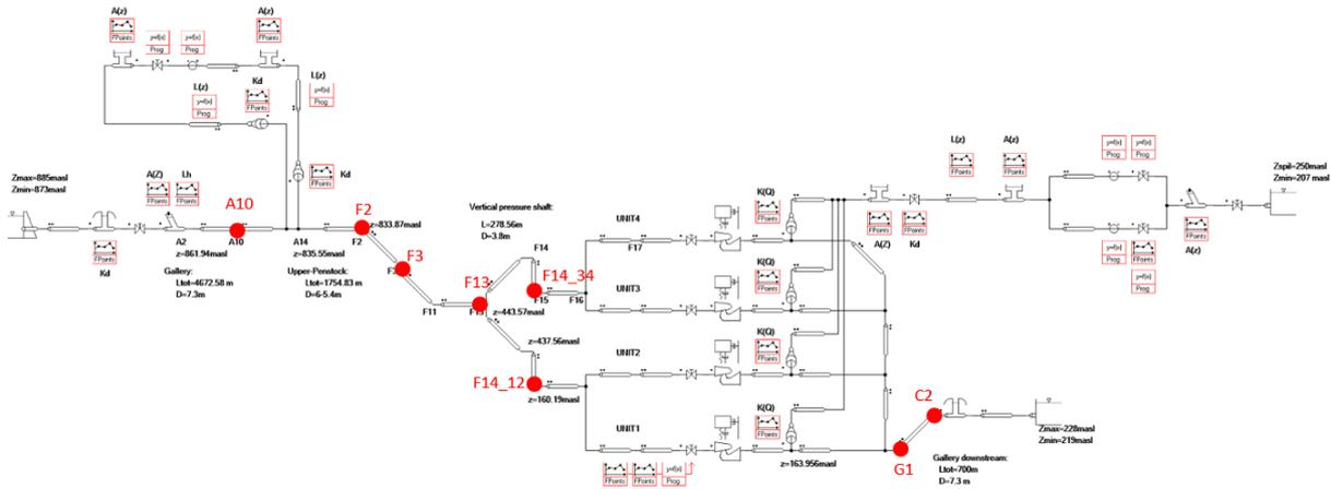
**Figure 4.** SIMSEN simulation model of the Gouvães PSPP.
