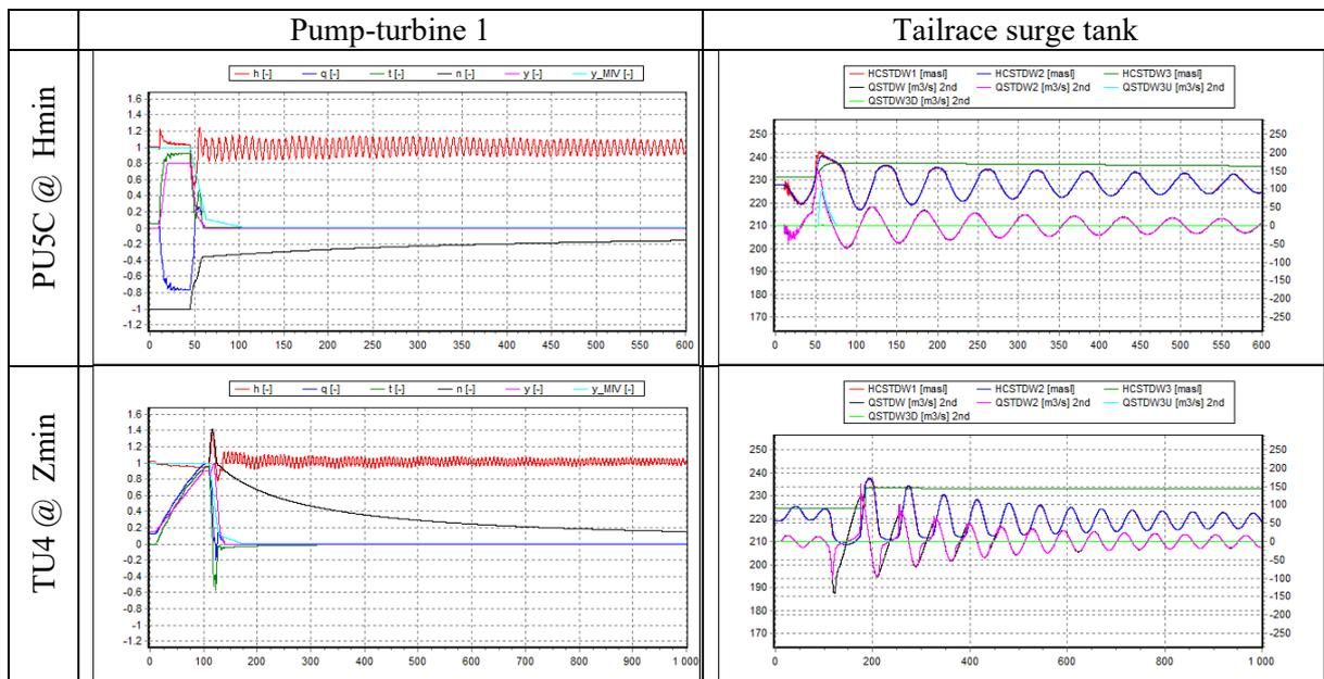
**Figure 6.** Numerical simulation results of the transient behaviour of the pump-turbine 1 and tailrace surge tank related to critical **normal** load cases for the tailrace surge tank maximum (top) and minimum (bottom) transient water levels.
