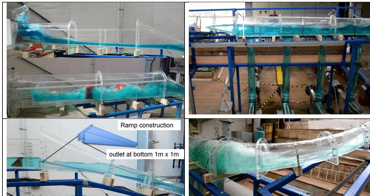
**Figure 10.** Gouvães tailrace surge tank transient flow achieved during physical transient model tests at TU Graz for the critical exceptional load cases related to up-surge in upper chamber (left) with ramp construction and down surge in the lower chamber and related risk of air entrainment (right), that was significantly mitigated by the ramp construction that creates a retention weir.
