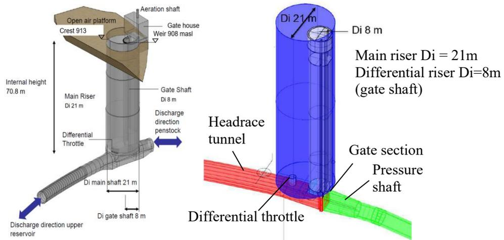
**Figure 2.** Layout of headrace differential surge tank of the Gouvães PSPP.
